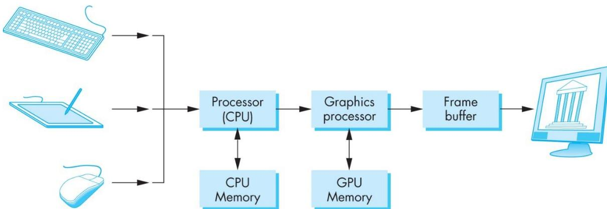
Most modern graphic systems are **raster-based** since the screen display is an array of pixels (picture elements). Each pixel corresponds to a location on the screen. Pixels are stored in part of memory called the **frame buffer**.
