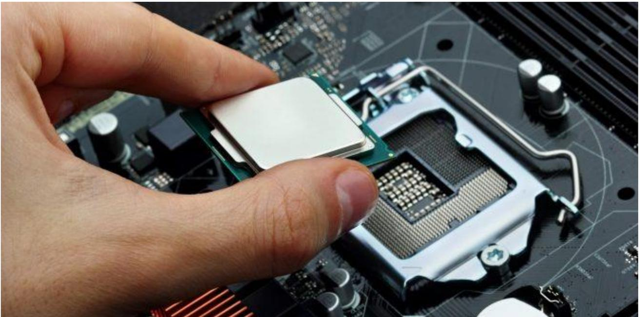
A CPU being placed in its socket
