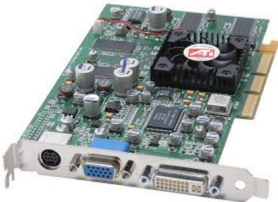
Unlike earlier graphics standards for PCs (MDA, CGA, and EGA) VGA uses analogue signals rather than digital signals. Consequently, a monitor designed for one of the older standards will not be able to use VGA.
