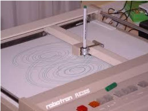
Pen plotters are still the most affordable printing device for CAD use and offer resolution unlike any other printer. The lines are not made up of dots. They are actually drawn, providing infinite resolution. There are a number of different types of plotters.
