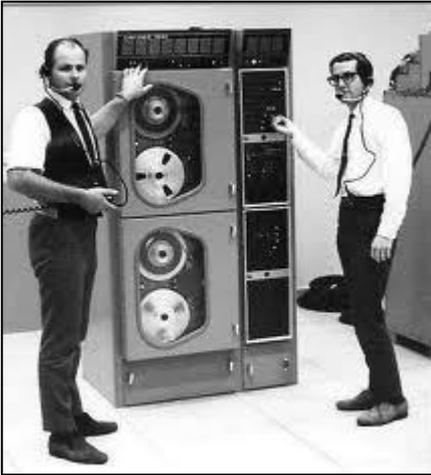
Tape has been more economical than disks for archival data, but that is changing as disk capacities have increased enormously. If tapes are stored for the duration, they must be periodically recopied or the tightly coiled magnetic surfaces may contaminate each other.
