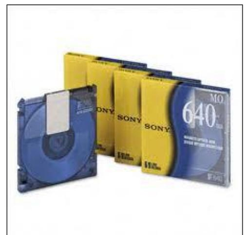
MO discs come in 3.5" and 5.25" cartridges. The latter are double sided, but must be removed and flipped over. Capacities of 3.5" cartridges vary but can hold up to 1.3GB. 5.25" disks can hold up to 9.1GB.
