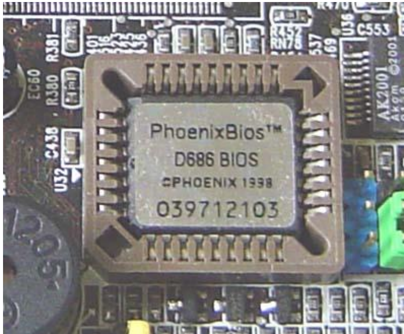
A CMOS ROM chip containing the BIOS
